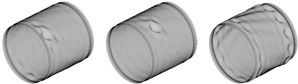
a) Mean imperfection \mu_w , time = 0.0011 s, P/P_{cr} = 0.918 b) \mu_w + \sigma_w imperfection, time = 0.0012 s, P/P_{cr} = 0.855 c) \mu_w - \sigma_w imperfection, time = 0.0010 s, P/P_{cr} = 0.943
